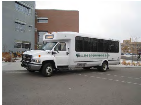
Figure 12. Cheyenne area fixed route transit service vehicles have front racks capable of carrying two bikes.
